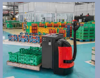
The support arm lift capacity is 2000 kg while the mast lift capacity is 800 kg
