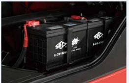
The battery is located above the fuel tank, there's battery box and adiabatic plate between them to prolong the battery's workling life.
