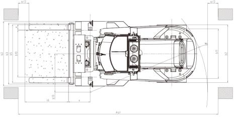
Ast=I6+Wa+x+a L6: load length a: Clearance (200mm)
